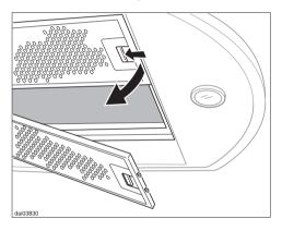
Remove the grease filters.
